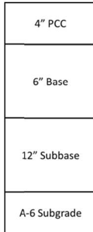
**Figure 1: Concrete pavement system defined as the control case P.**
